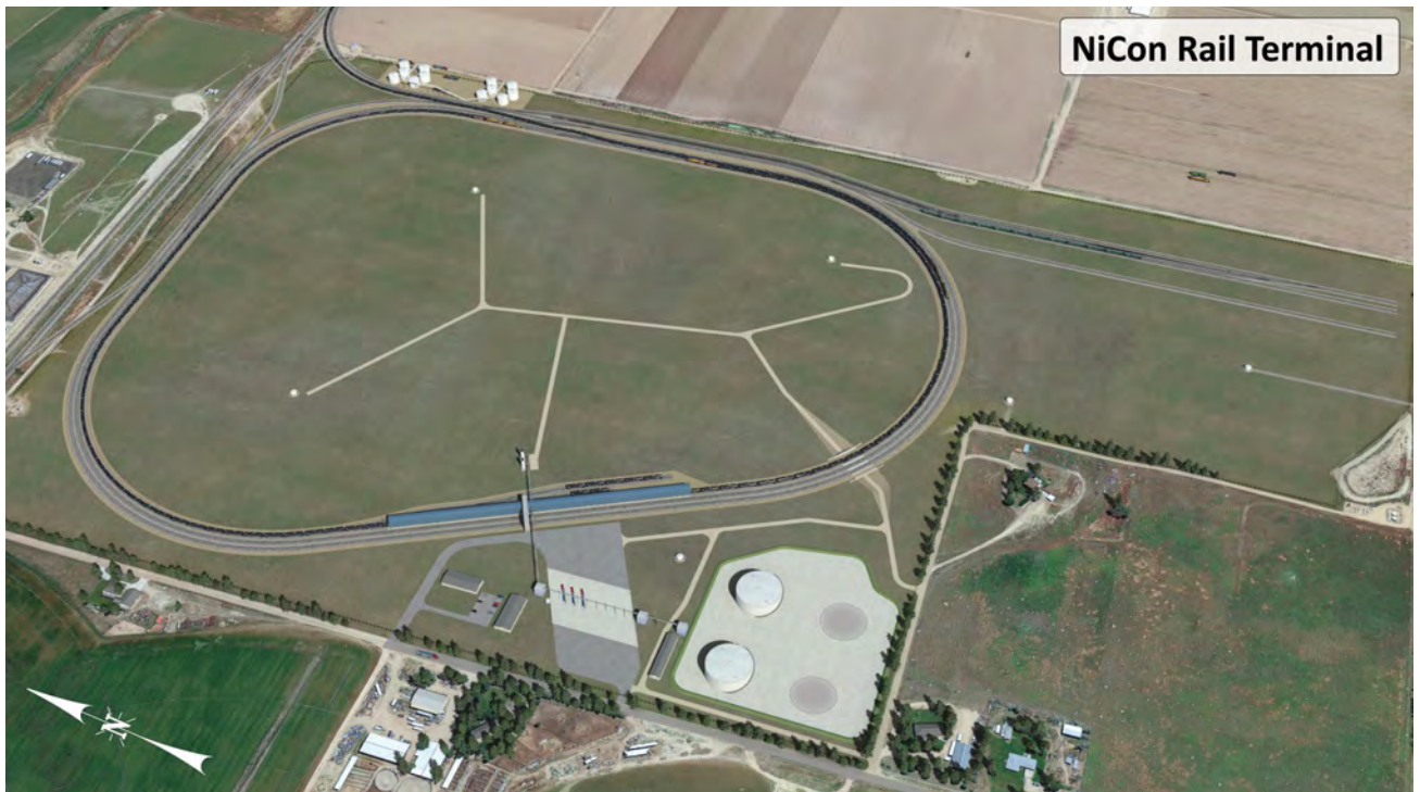
The Niobrara Connector will help balance the Denver-Julesburg Basin market by providing inbound capacity for frac sand and drilling materials as well as outbound for crude and liquids production. This rendering shows the facility, in the heart of the play, from above.
